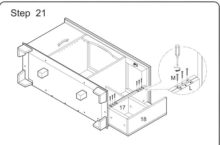
Attach door assembly (17,18) to the opposite side of the stand assembly at door hinges (L) using large screws (M).
